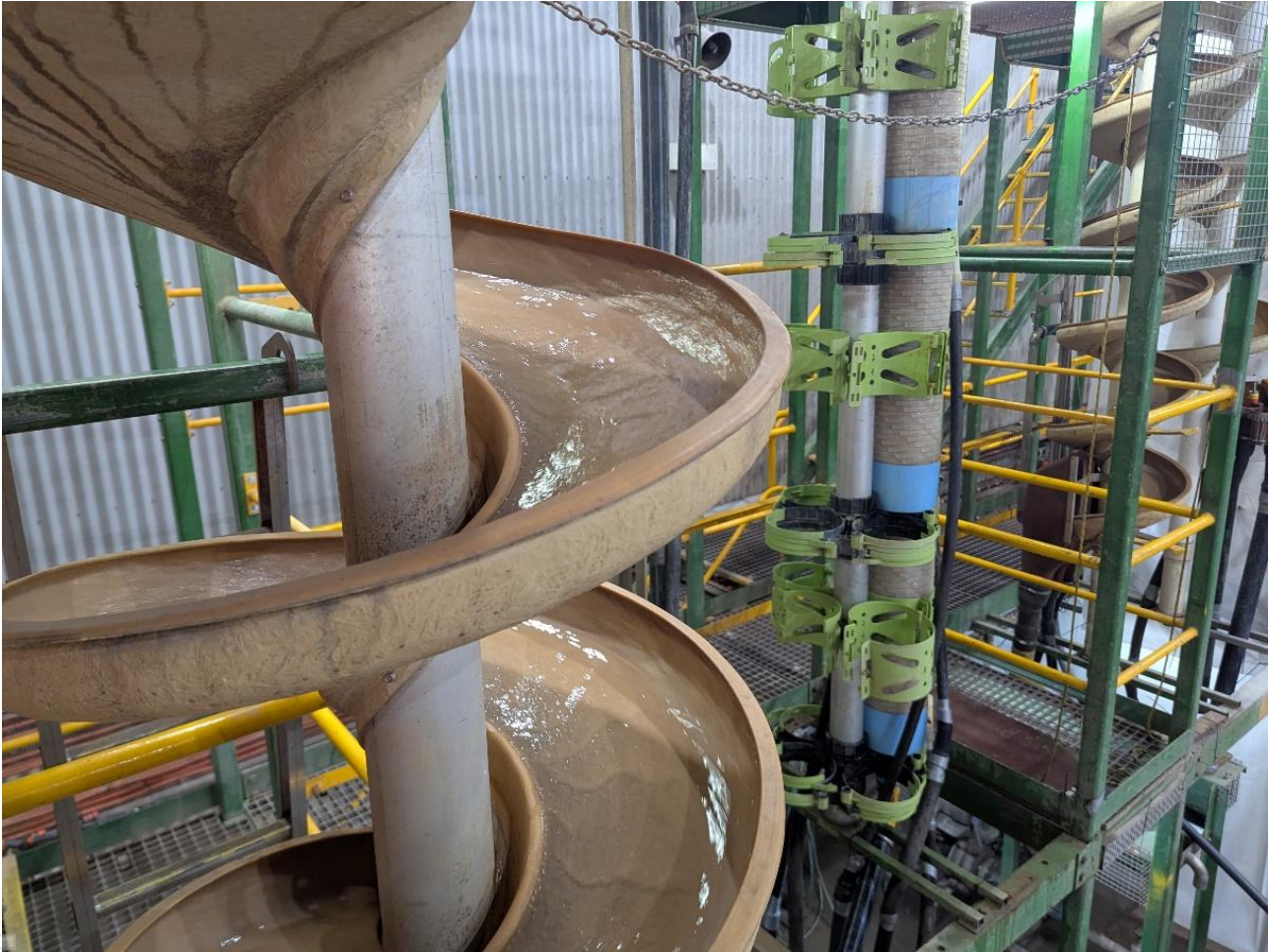
Figure 1: MG12 spiral foreground & CT1 spiral background (fully enclosed small diameter)
