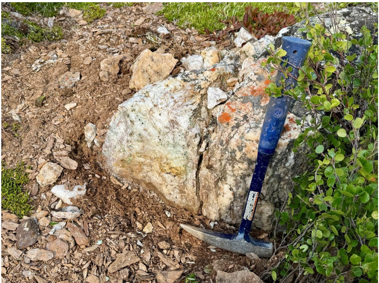
Figure 3: | Rock sample M209513, quartz vein outcrop at the southwestern end of the Jaws target which returned 3.25g/t Au, 15.3g/t Ag, 1.185% Cu and 0.885% Sb.
