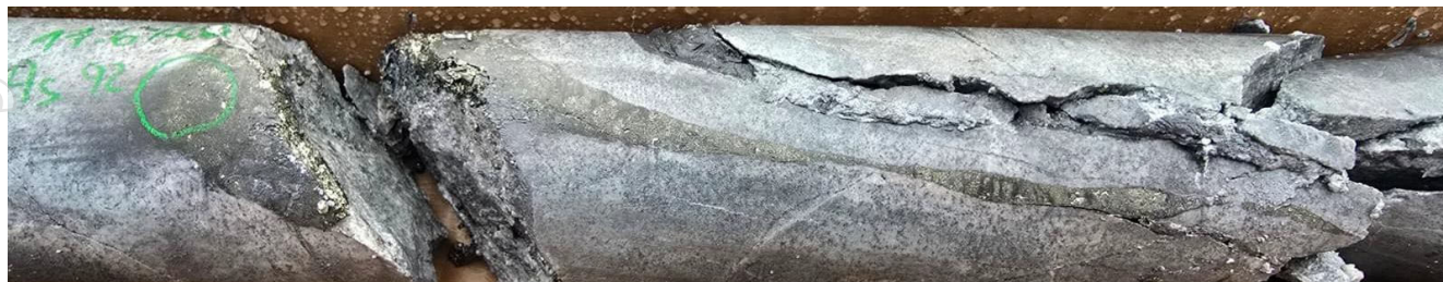
Photo 2. Chalcopyrite (Copper) sulphide within a c-type vein within altered porphyry in 25LLDD0070 from 400m*.
