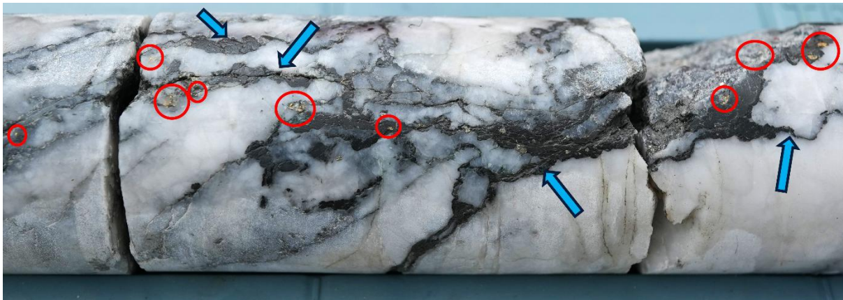
Figure 8 BMDD001W6 showing visible gold (red circles) and stylolites (blue arrows) in the NQ core (47.6mm diameter) from 832.7 to 832.9m
