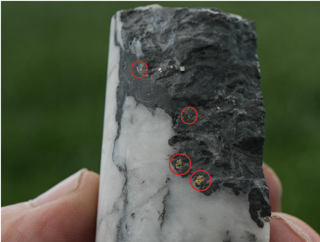
Figure 11 Visible gold in NQ core (47.6mm diameter) in BMDD001W6 at 832.9m
