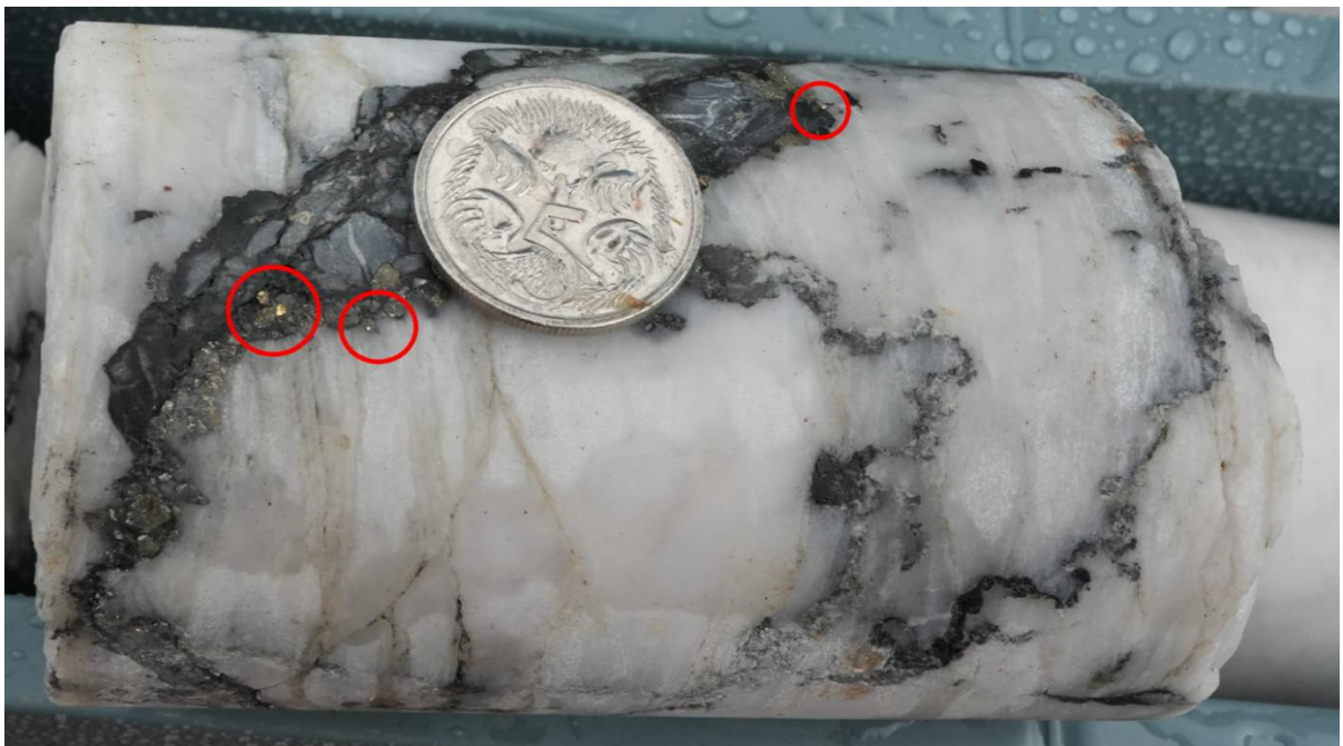
Figure 9 BMDD001W6 showing visible gold (red circles) in the NQ core (47.6mm diameter) from 834.8m
