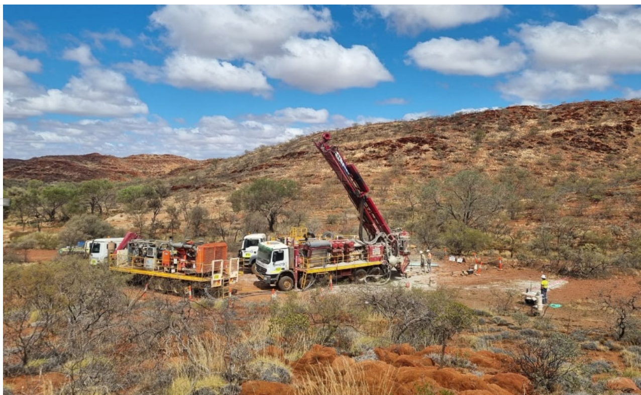
Figure 1: RC drilling one of 2 lodes already identified at Big Sarah.
