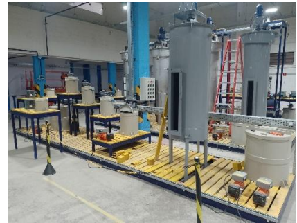
Figure 4: Impurity removal circuit
