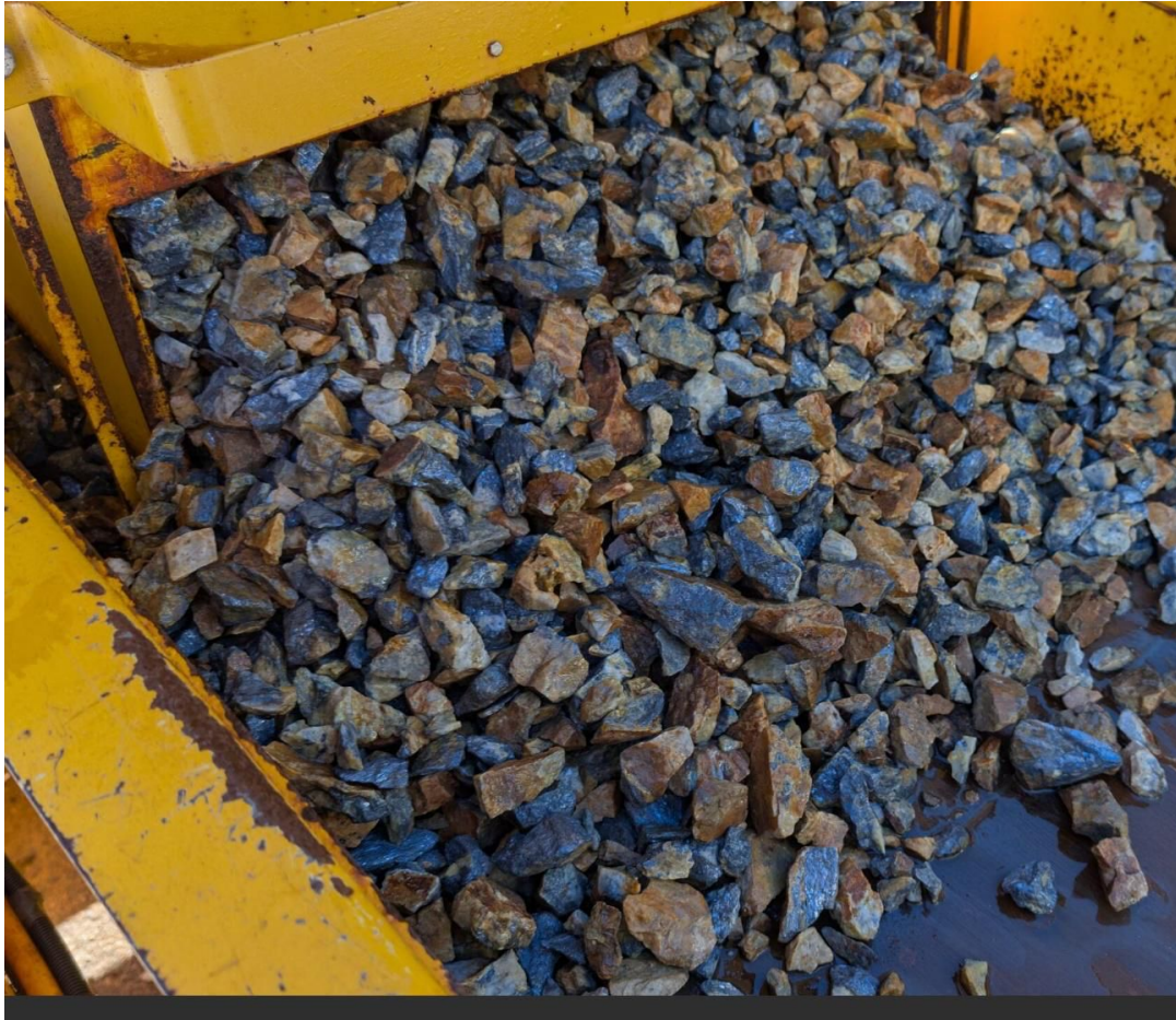
Figure 7. Ore sorted material from a single pass grading 49.1% antimony trisulfide (35.2% Sb)
