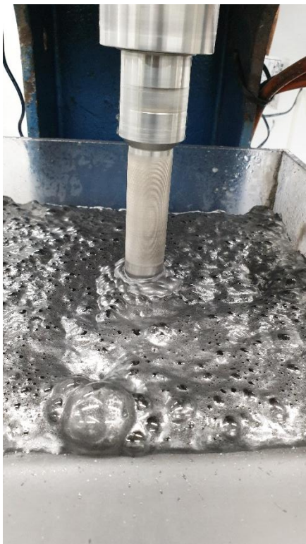
Figure 17: Copper concentrate from Nyungu Central transition composite – chalcocite is the major copper mineral
