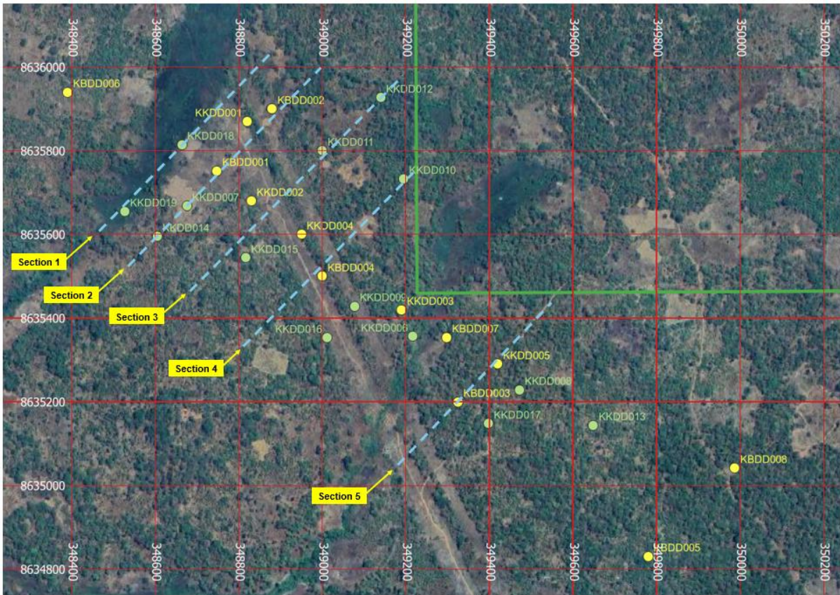
Figure 7: Kabikupa drill hole collar plan showing Prospect Phase 2 drill holes (green), pre-2025 holes (yellow) and oblique drilling cross sections described in this release (as dashed blue lines)
