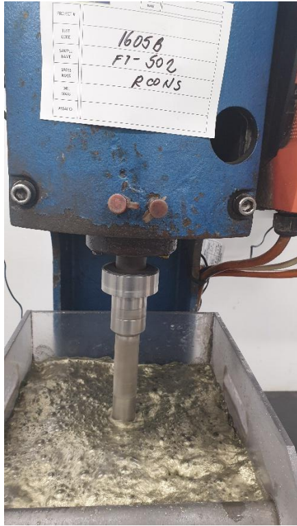
Figure 16: Copper concentrate from Kabikupa fresh composite – chalcopyrite is the major copper mineral
