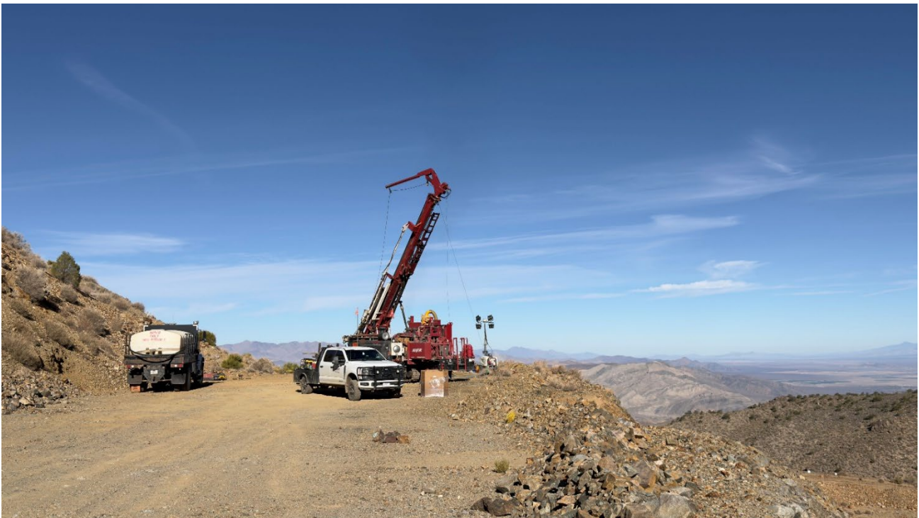
Figure 1: RC rig infill drilling the North Pipe at Colosseum
