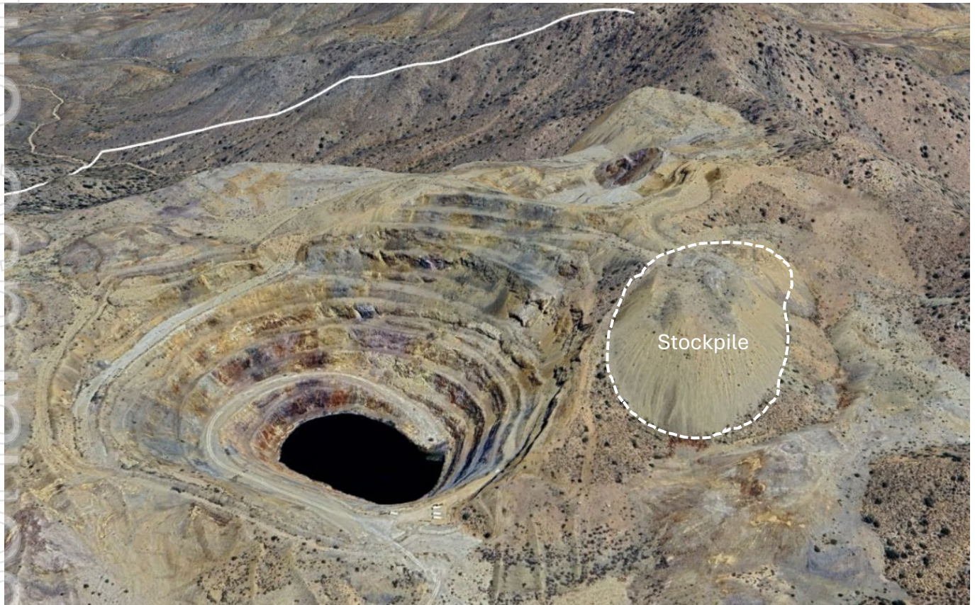
Figure 2: Stockpiles to be assessed with RC drilling
