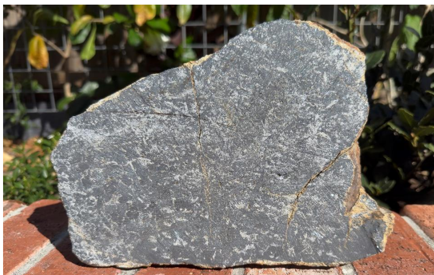
Figure 4: Photograph of rock sample TJ25ROC4 showing the massive Stibnite mineralisation (sample is ~20cm across)
