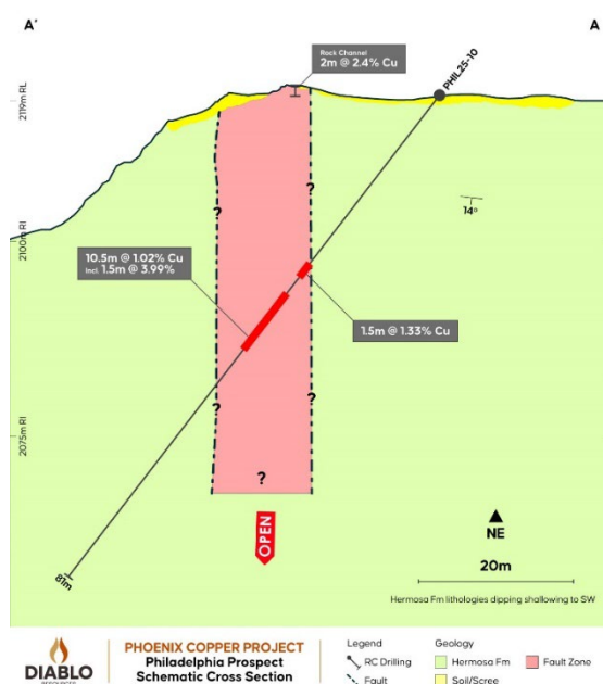
Figure 3 – PHIL 10 Schematic Cross Section
