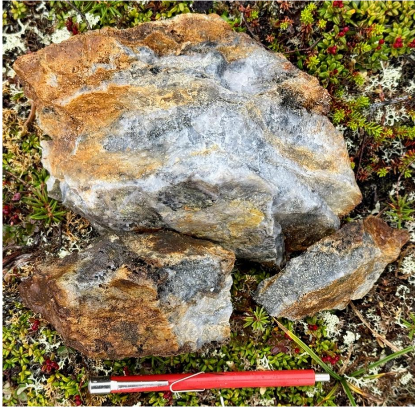
Figure 4: I Rock sample M209523 from the Lotus target area. Sample returned 8.01g/t Au & 2660g/t Ag .
