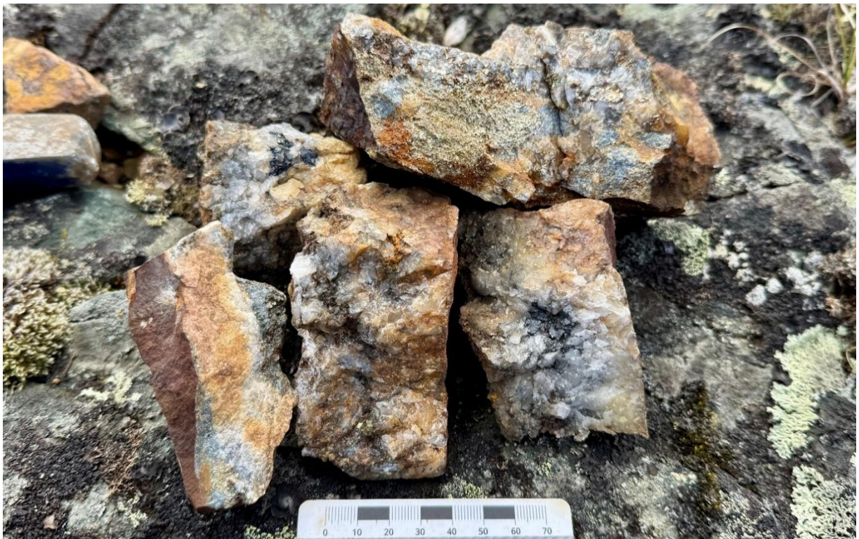
Figure 3: | Rock sample M209538 from the Quantum target area. Sample returned 14.05g/t Au , 1385g/t Ag , 0.32% Cu .
