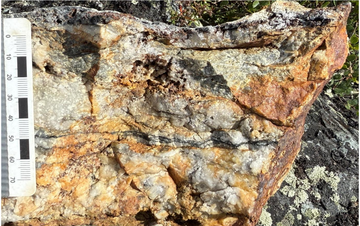
Figure 2: | Rock sample M209533 quartz vein from the Quantum target area. Sample returned 16.75g/t Au and 385g/t Ag .
