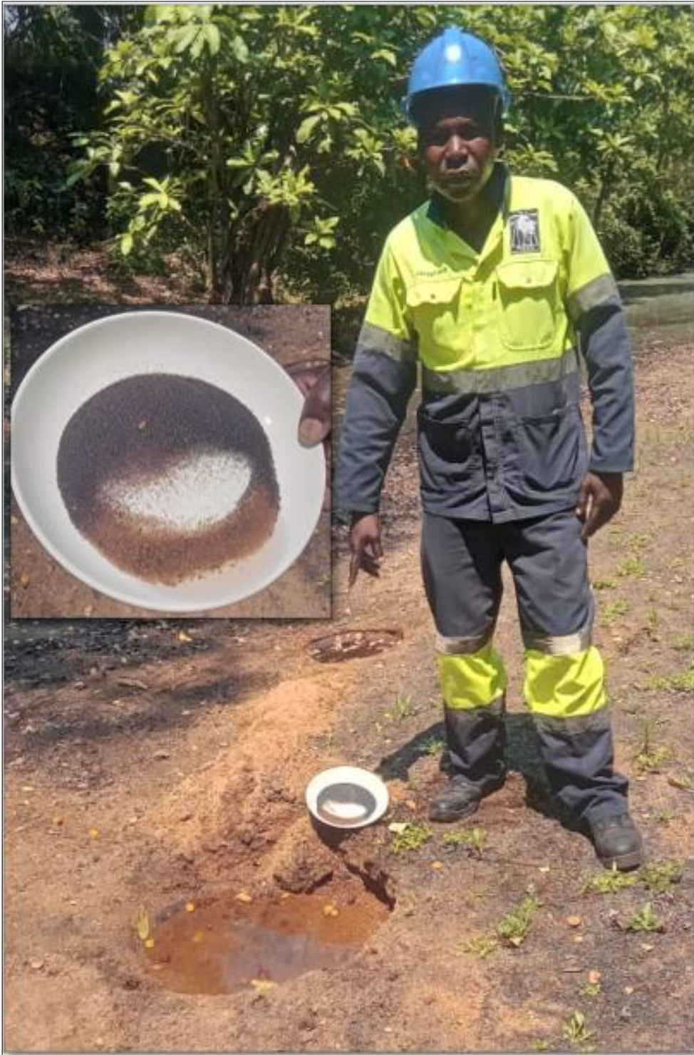
Figure 2: Very high concentration of Heavy Minerals within the stream seen near stream sedimentary sampling point 2402SED042 within Adriano (11002L).
