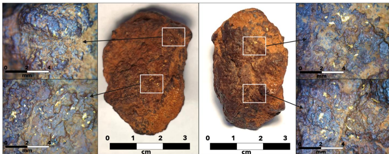
Figure 3: Rock specimen found containing abundant gold. Picture shows both sides of the specimen and close up images of showing the gold occurring throughout the sample. Grade cannot be estimated from visual abundance.
