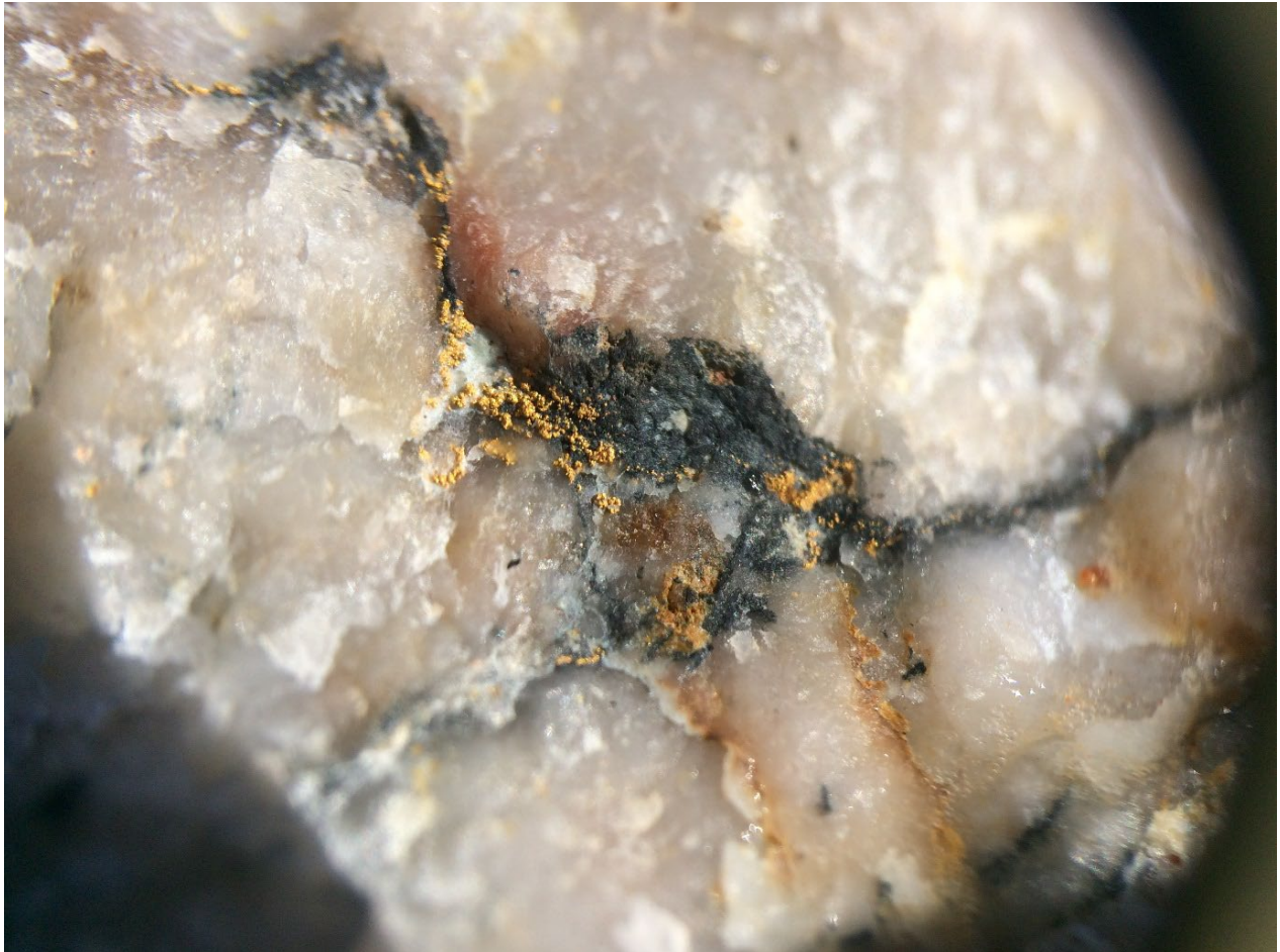
Plate 3: Visible gold along darker sulphide rich stringers in laminated quartz vein
