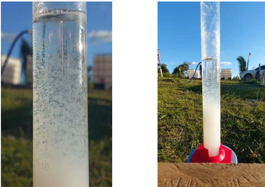
Figure 1. Precipitated solids directly in the field after in-situ leaching. Small amounts of reagent added to rare earth rich solution causing the rare earths and impurities to precipitate (cloudy material) in a beaker directly adjacent to extraction wells.
