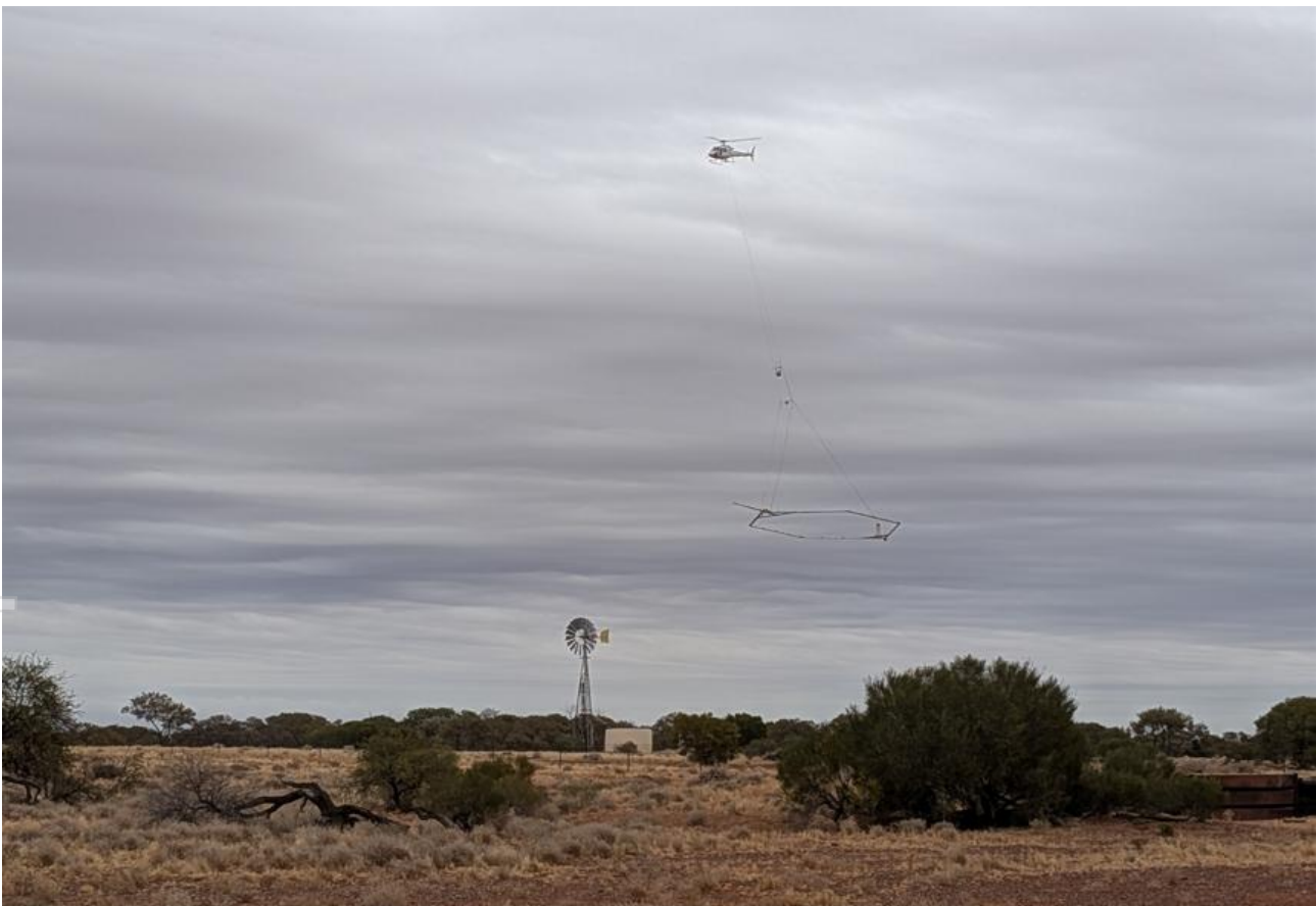
Figure 9 – Helicopter acquisition of high-resolution SkyTEM Airborne EM survey data over the Marymia East project.
