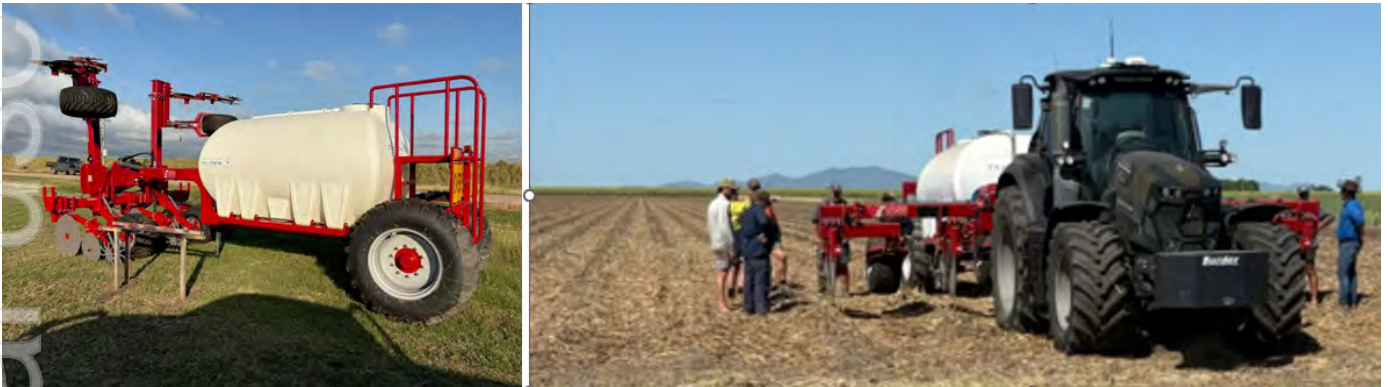
Figure 3: RLF Liquaforce variable-rate liquid applicator ready for first use in Ayr, Queensland (left). North Queensland growers discussing the applicator's first run (right).
