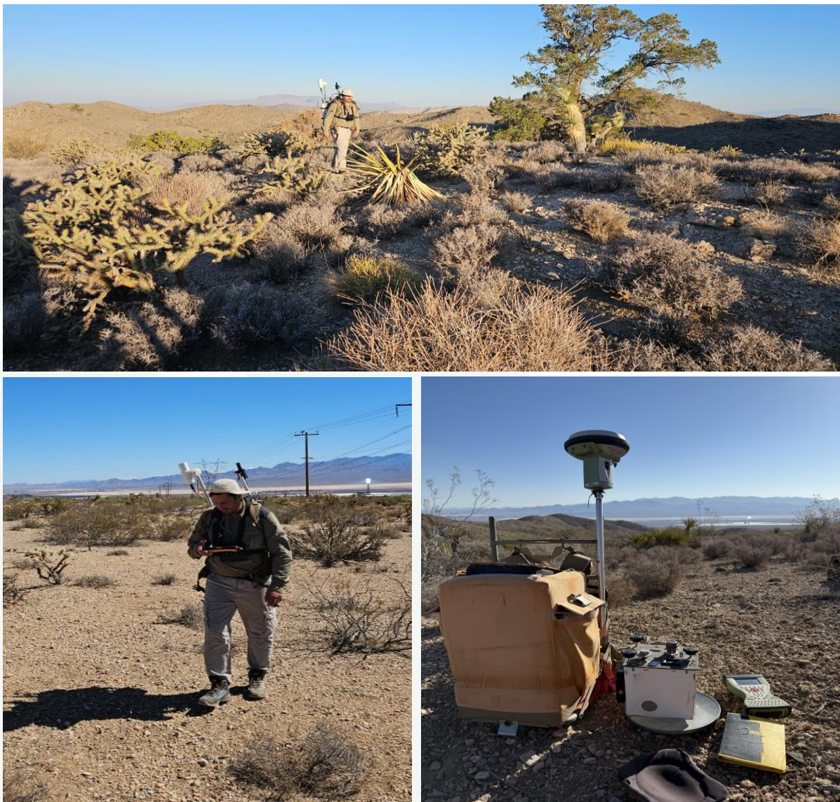
Figure 6: Field crew conducting ground magnetic and gravity survey at Desert Star Project
