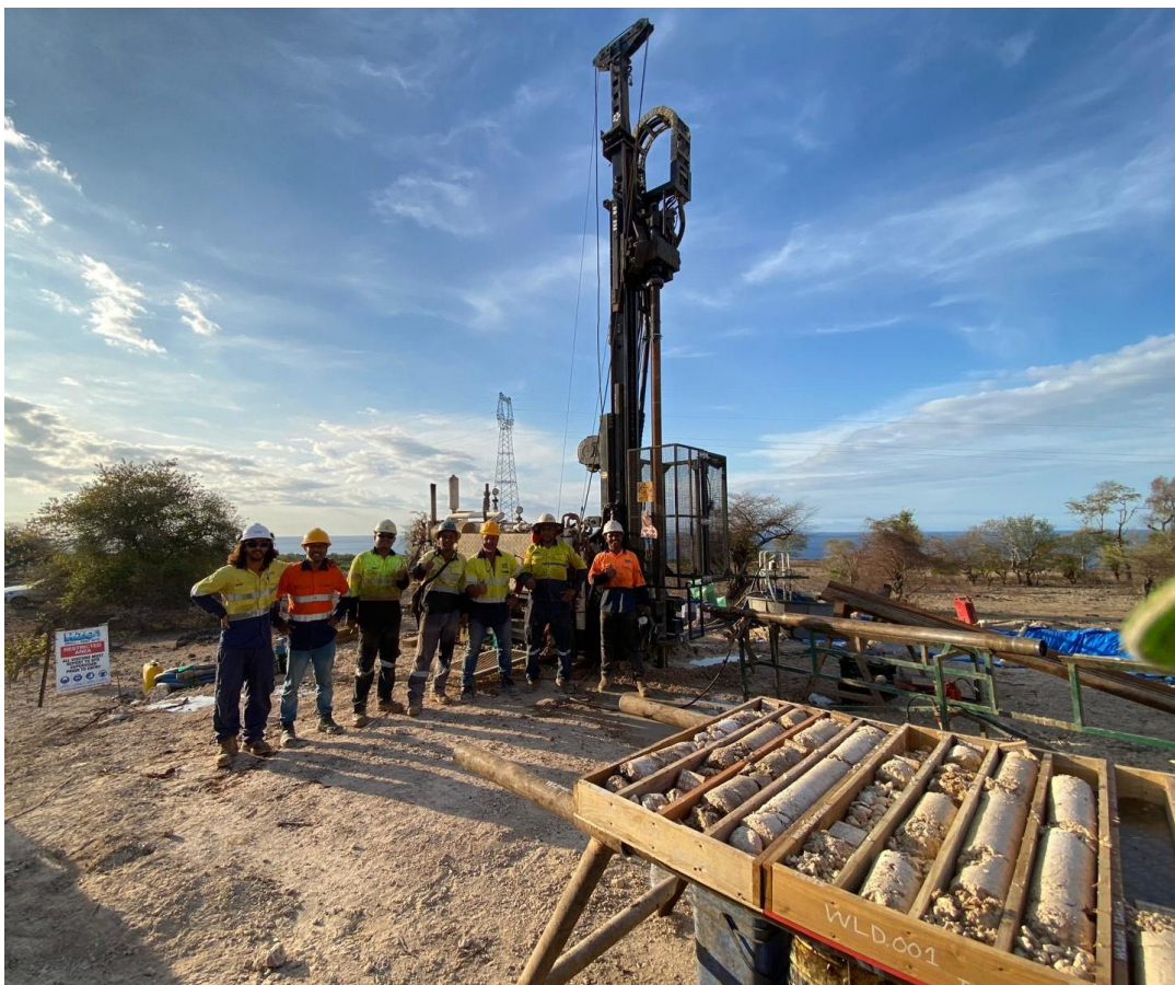
Figure 1: Collaring of the first diamond drillhole WLD001 at the Werumata Limestone Project with Estrella's exploration team and Coresearch drill team.
