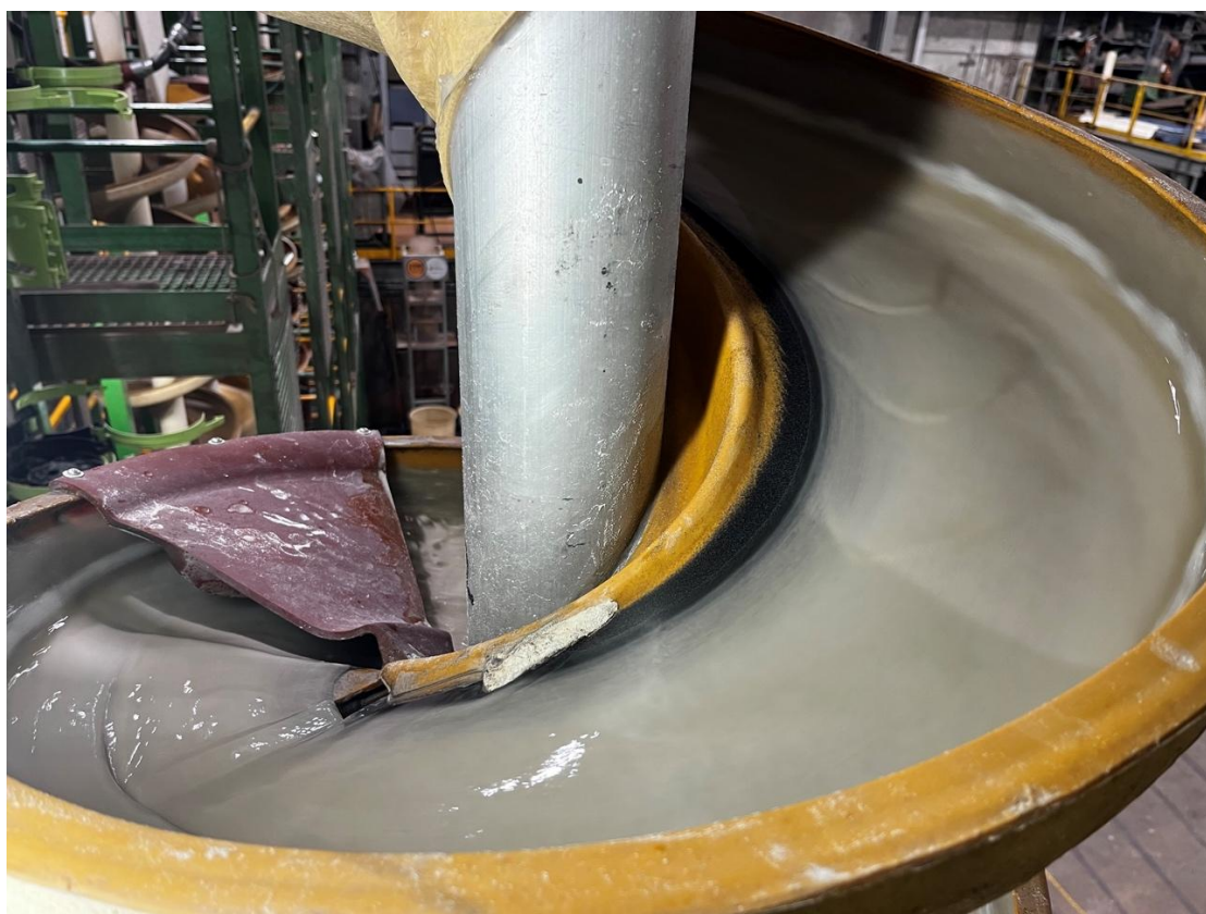
Figure 3: Spiral separation of bulk metallurgical testwork from the NSP
