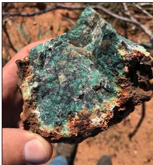
Figure 8: Quartz-chalcocite filled vugs in Cromwell A shear zone with malachite rosettes ( \pm 5\text{-}12\% visual est.) intergrown with chalcocite ( \pm 2\text{-}4\% visual est.)
