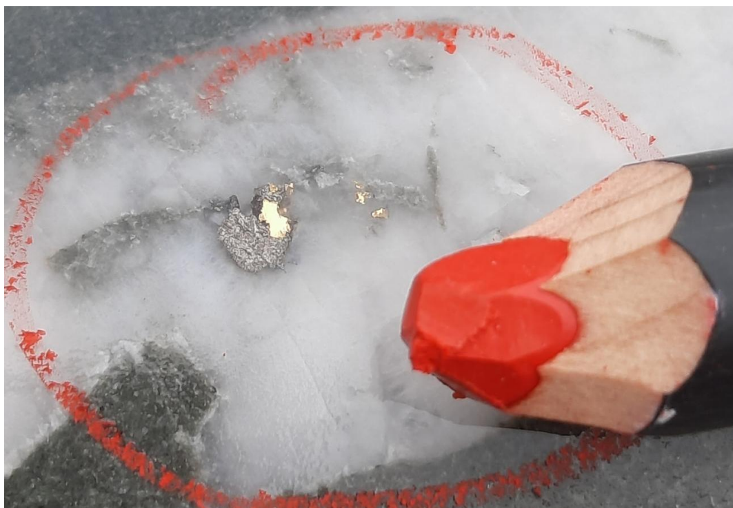
Figure 1. Visible gold 1 grains (lustrous yellow) up to 2mm associated with sulphides (grey) in quartz from AMD014A at 465.0m. Assays are currently pending for this hole.
