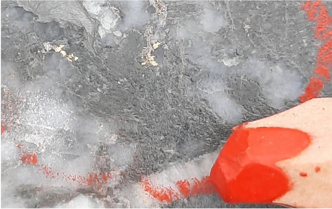
Figure 4. Multiple patches of visible gold 1 up to 2.5mm (lustrous yellow) within an irregular quartz stockwork zone in hole AMD014A at 466.0m. Assays are currently pending for this hole.
