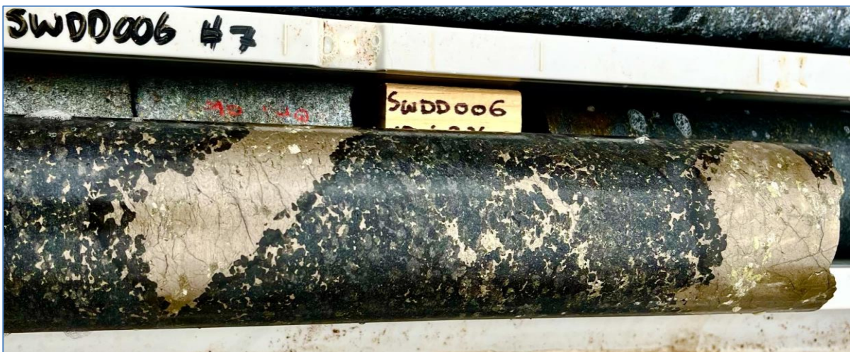
Figure 1. Drill core from hole SWDD006 (226.55 – 226.85 m) showing net-textured to semi-massive magmatic sulfide mineralisation composed predominantly of pyrrhotite, pentlandite, and chalcopyrite.
