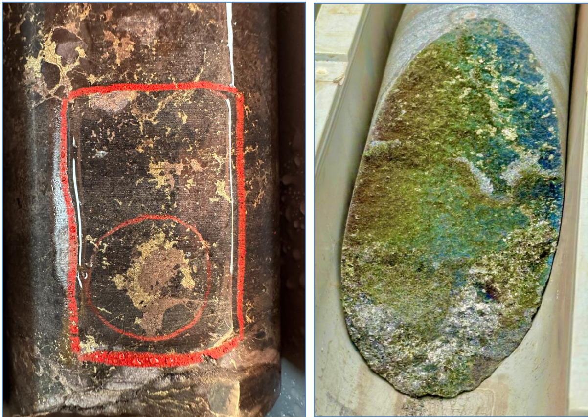
Figure 2. (Left) Net-textured chalcopyrite–pentlandite–pyrrhotite mineralisation in hole SWDD006 (226.55–226.85 m) showing interconnected sulfide networks within a magnetite-bearing mafic host, typical of magmatic segregation and coalescence of immiscible sulfide melt. (Right) Bornite–chalcopyrite sulfide band developed along a fracture plane in SWDD002 (86.7–89.42 m). Assays pending.
