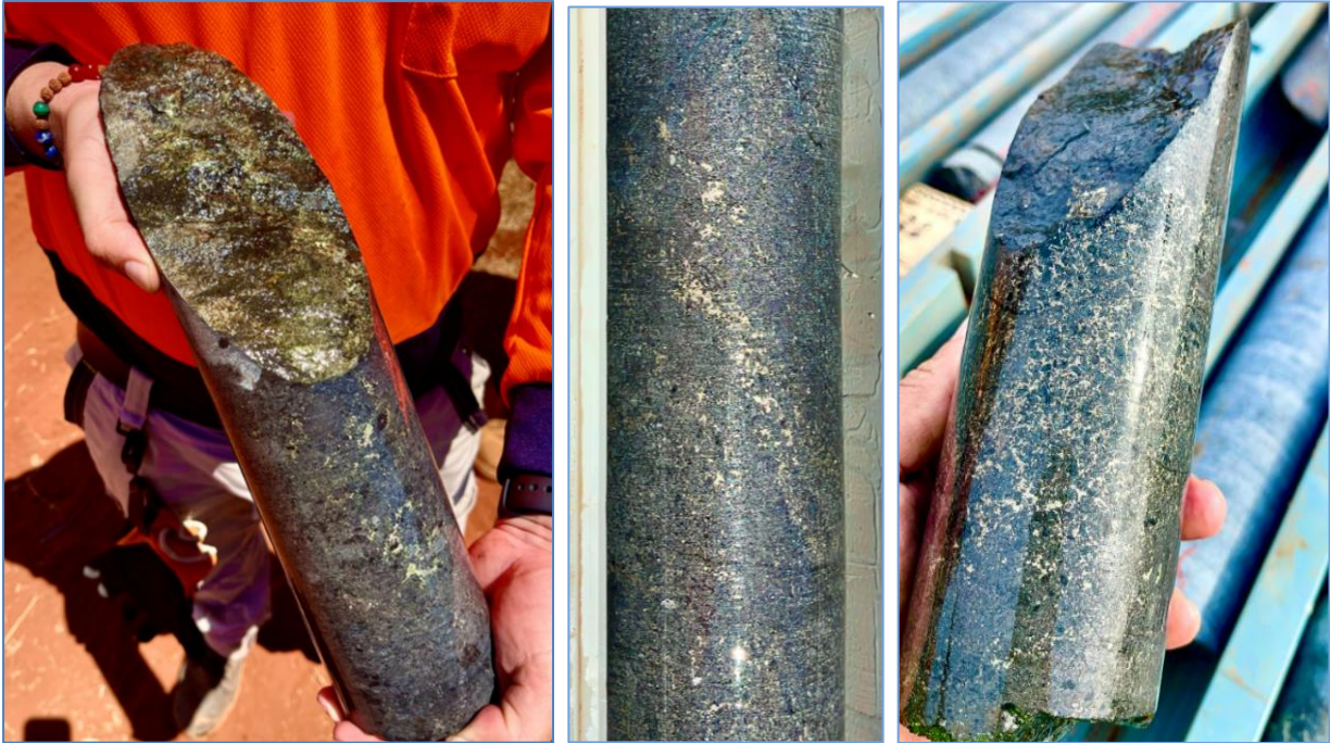
Figure 3. (Left to right) Chalcopyrite-rich fracture-fill vein and adjacent net-textured to globular sulfide mineralisation in drillhole SWDD003 (75.38–75.80 m); disseminated chalcopyrite–pyrrhotite–pentlandite sulfides in SWDD003 (200.1–200.6m); and net-textured magmatic sulfides in SWDD002 (110.3–110.7m). Assays pending.
