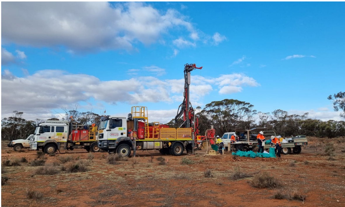
Figure 3: Air Core drilling at EL 6895.
