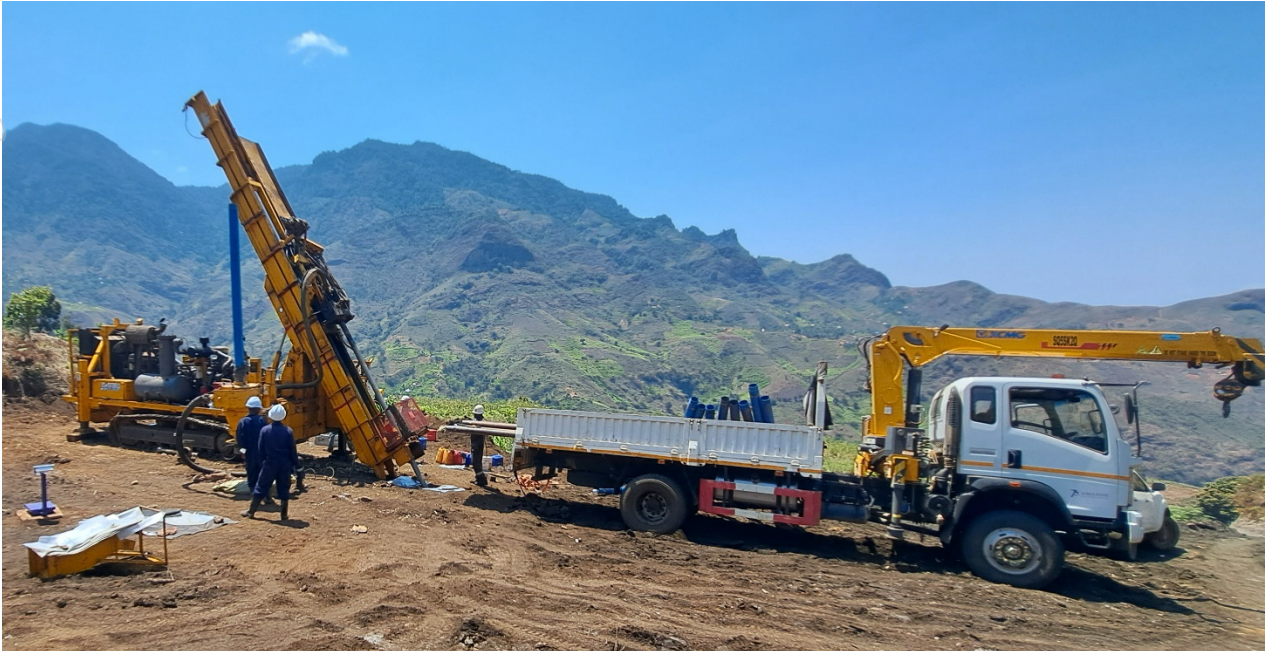
Figure 2: RC drill rig in operation at Kumba Deposit, Morogoro Graphite project, Tanzania. Drilling has commenced adjacent to trench TRUM23-002.
