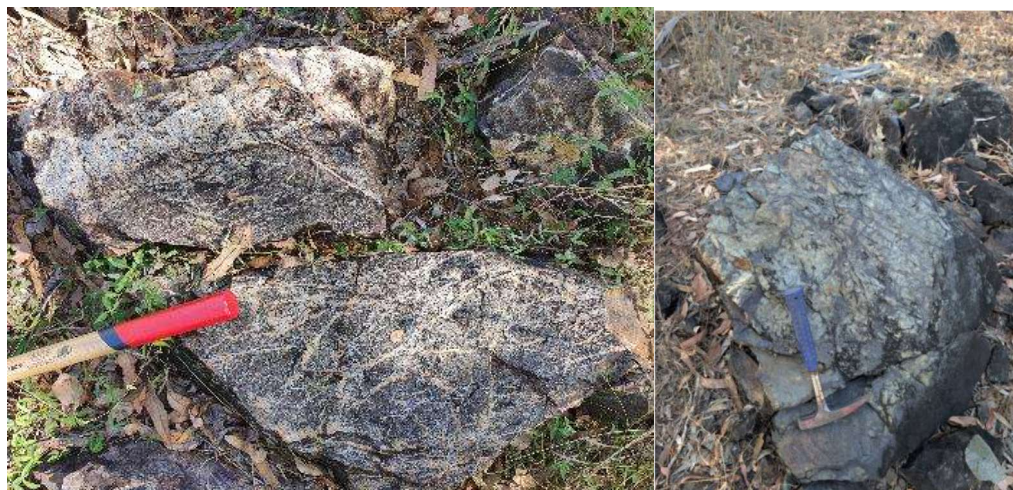
Figure 8 – Outcropping geology from the Megan Veins target area. Left - Epithermal style quartz stockwork veins with rock chip samples grading up to 10g/t gold 8 . Right – Strongly hydrothermally altered diorite outcrop.
