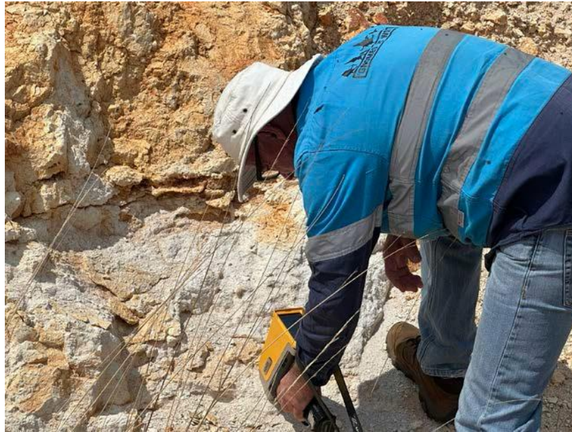
Figure 13. REE Target - pXRF sampling of white weathered kaolinitic fine-grained sediments adjacent to the prominent scarp as shown in Figure 12
