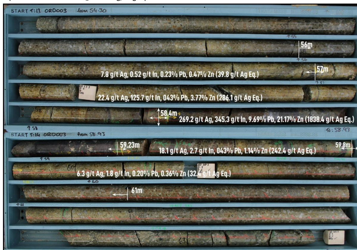
Figure 3 Orient West Diamond Drilling (ORD003) – 5m @ 428.6 g/t Ag Eq. from 56m inc. 2.8m @ 737.3 g/t Ag Eq. from 57m inc. 0.83m @ 1838.4 g/t Ag Eq. from 58.4m
