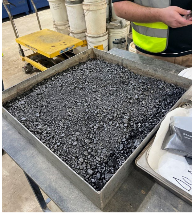
Figure 3: Graphite concentrate (93.4% graphite) sample used in purification tests 3
