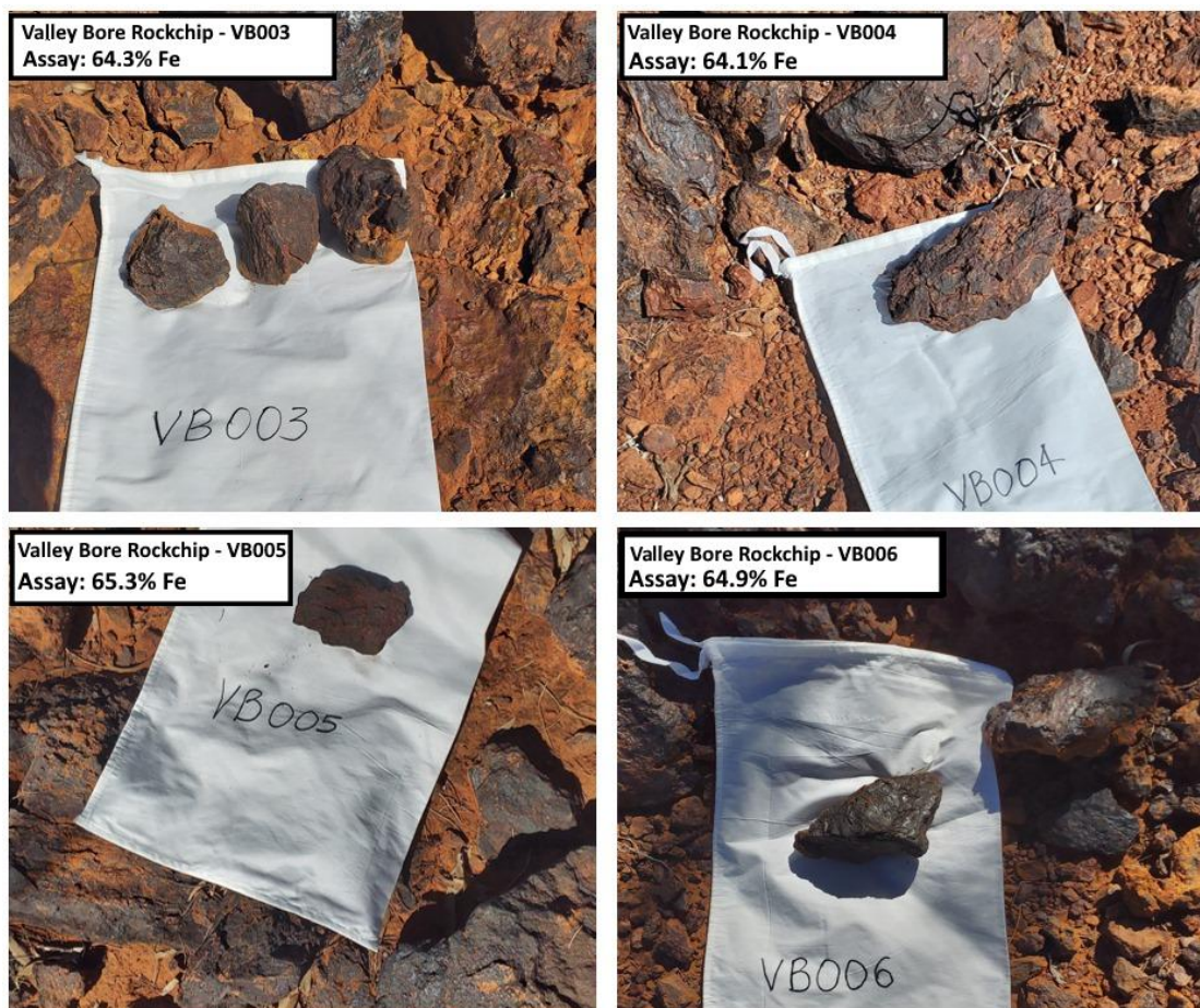
Figure 8: Rock chip samples with assay results from Valley Bore Southern Ridge target (results in % Fe) 9
