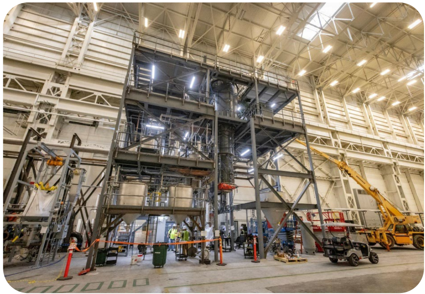
Figure 2 Mass production furnace at Riverside facility.
