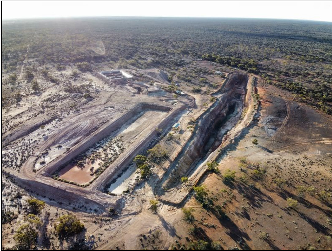
Figure 4: Drone photo of Zelica Project looking NNW showing pre-stripped open pit (approx. 300m long and 10-25m deep) and pre-constructed vat leach ponds (pic taken August 2025)
