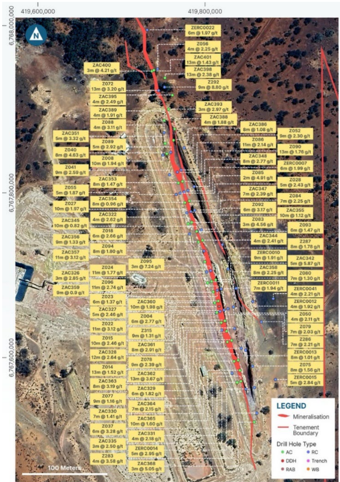
Figure 5: Aerial Photo of Zelica Trial Pit with Drilling and Projection of the Gold Mineralisation along approximately 300m of the ~1km mineralised strike 4
