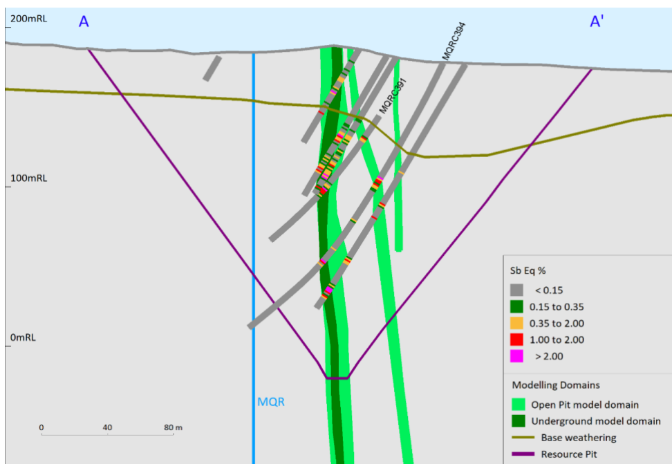
Figure 5 – A-A' section view facing east with open pit and underground domains illustrated with projected one metre downhole assays. Conceptual MQR open pit shell also projected onto section.
