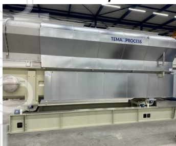
Fluid bed dryer built
