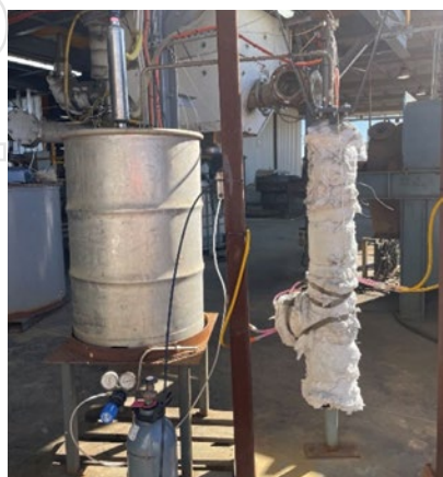
Figure 2 – (L–R) Vertical kiln prototypes, pyrrhotite product after pyrite conversion and sulphur collection in condenser
