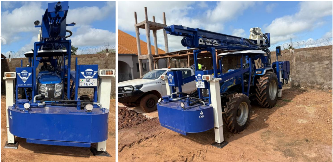
Figure 3: Tractor-mounted auger drilling rig
