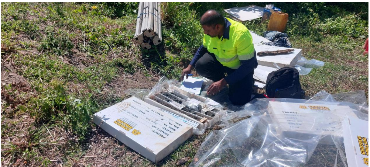
Plate 3 – Sand core samples being logged and packaged for shipment to the laboratory
