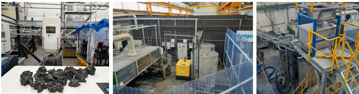
Pictures: (from left) Graphite concentrates from recycling partner; (centre and right) undergoing Talga's process into purified, shaped and coated anode material fit for re-use in lithium-ion batteries.
