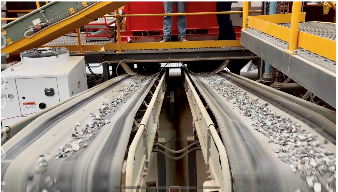
Figure 3. Ore Sorting Tests at the TOMRA Facility processing Tungsten ore from the Cleveland Project
