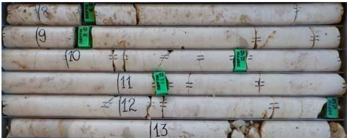
Fig 1 - Soalara Limestone Core - High purity @ 97% Calcium Carbonate
