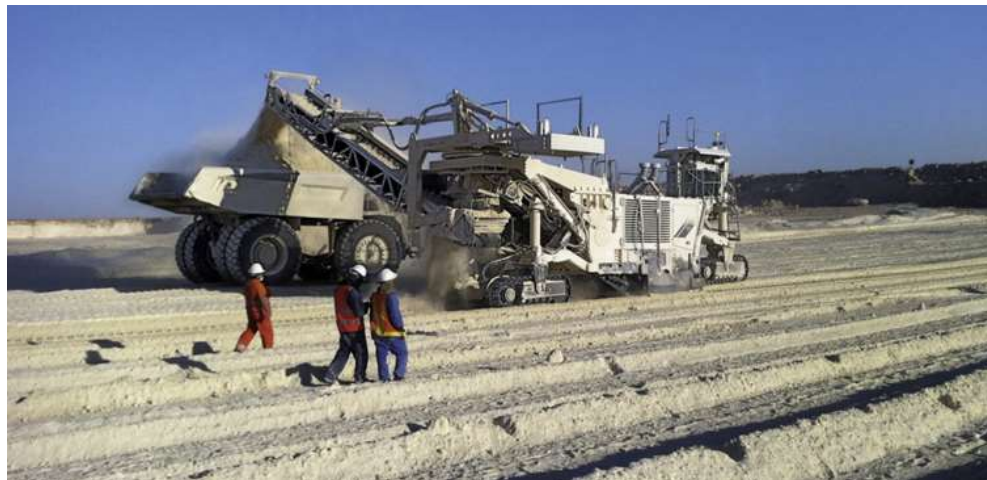
Fig 3 - Example Surface Miner – Limestone row cutting
