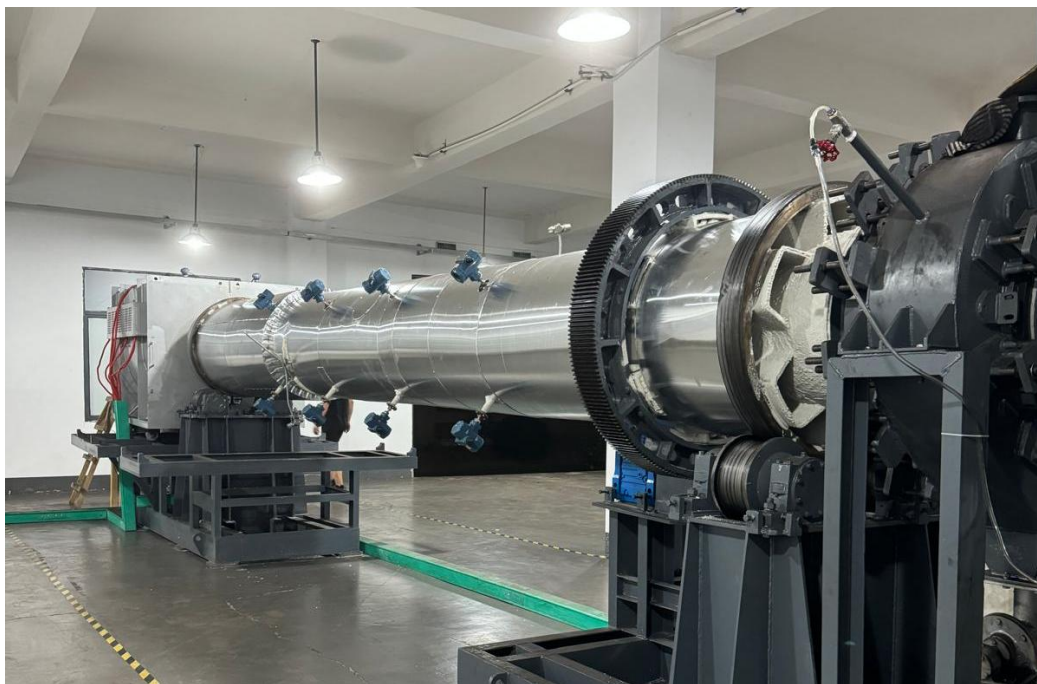
Figure 3: Firebird high efficiency demonstration calcination kiln
