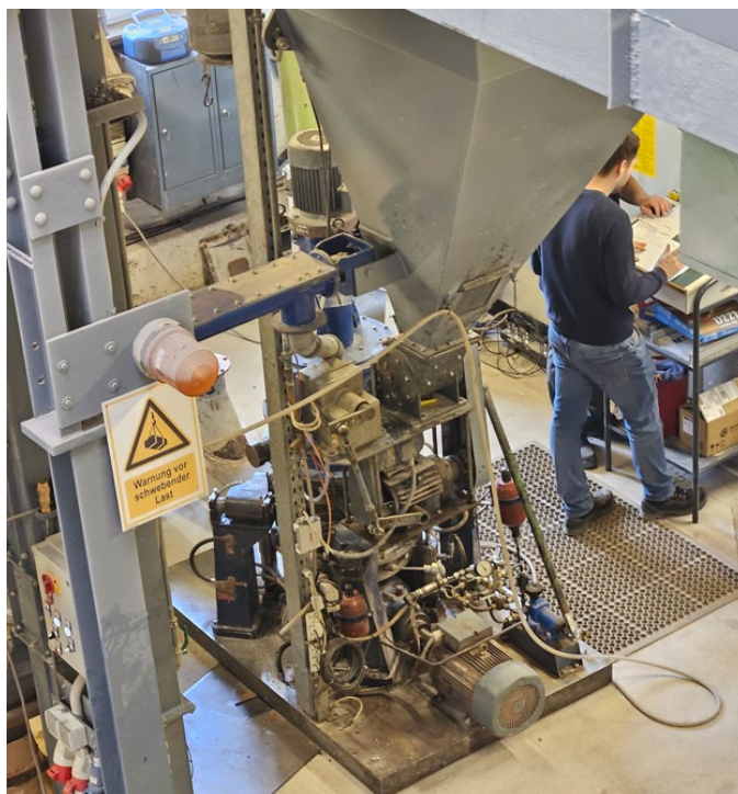
Figure 3: GEBR Pfeiffer VRM test facility
