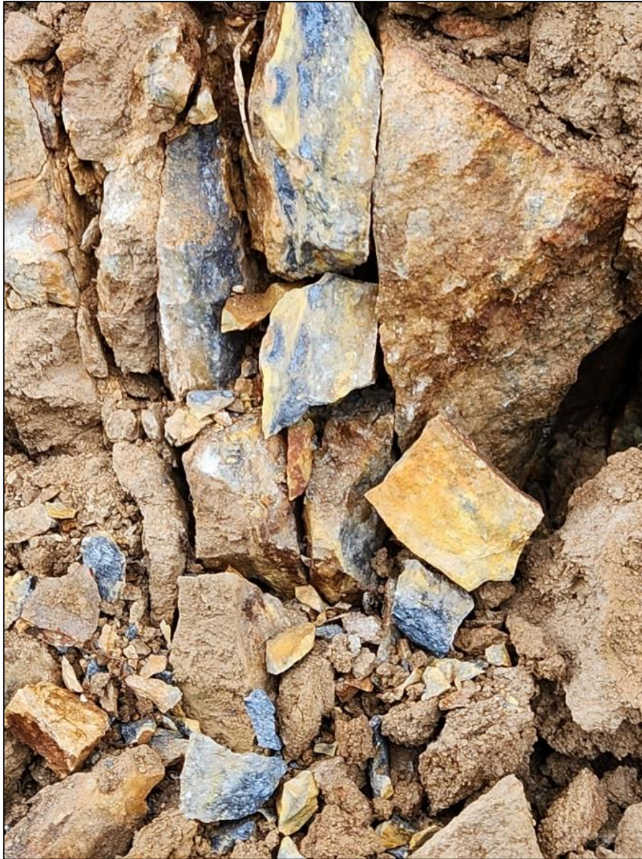
Figure 6: Trench wall photo looking west of antimony bearing sub-vertical vein, site of BSE008 sample.
