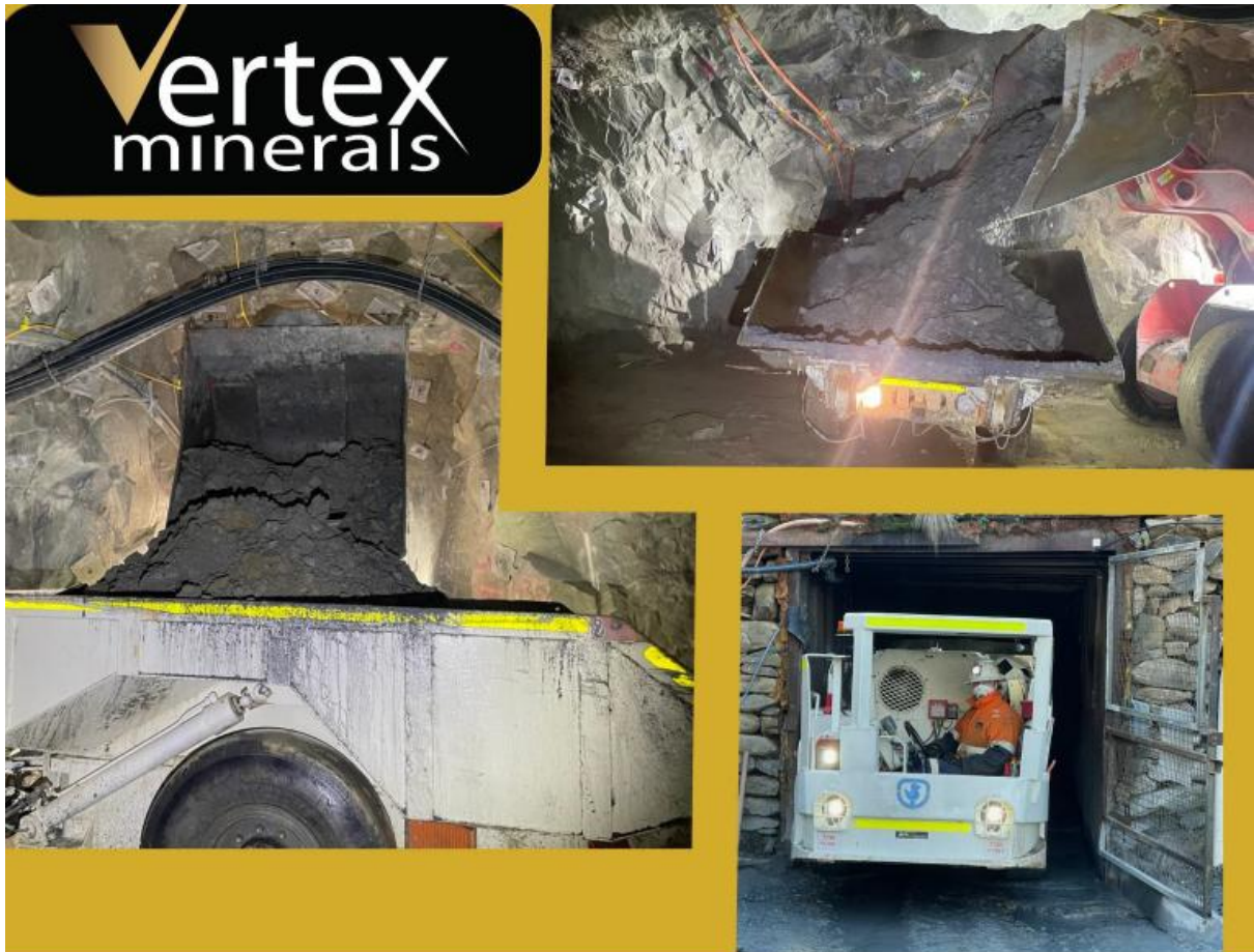
Image 5: Truck being loaded with ore and hauled to processing plant from the Lady Belmore Reef vein
