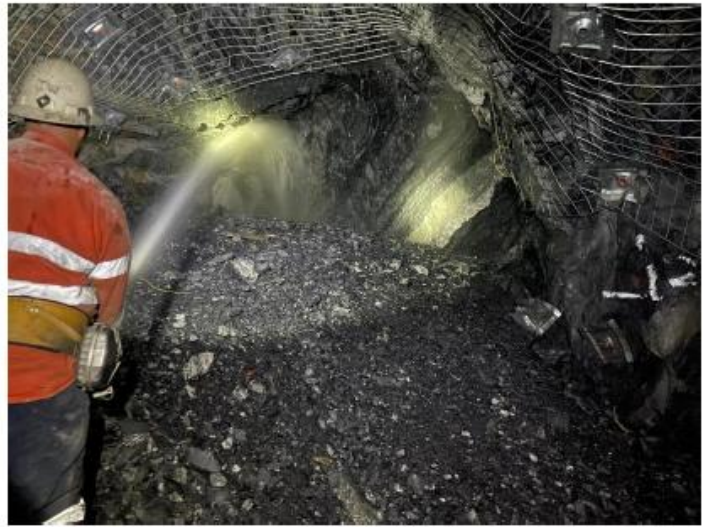
Image 4: Lady Belmore Reef being charged up and house down the ore, post blasting
