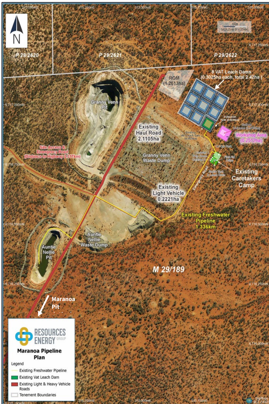
Figure 1: Maranoa Vat Leach Pipeline Plan
