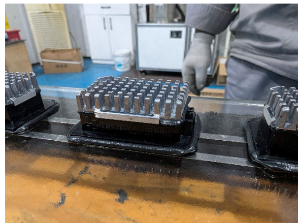
ClearVue patented thermal bridge single glaze junction boxes installed for testing.
