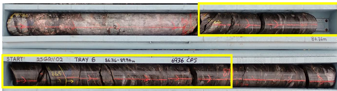
Figure 1 – Core from drill hole 25GRV002 with very high-grade interval @ 6,929.57ppm U 3 O 8 from 86m downhole.
