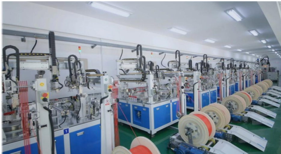
Figure 1: Automated Production Line for Electronic Detonators
