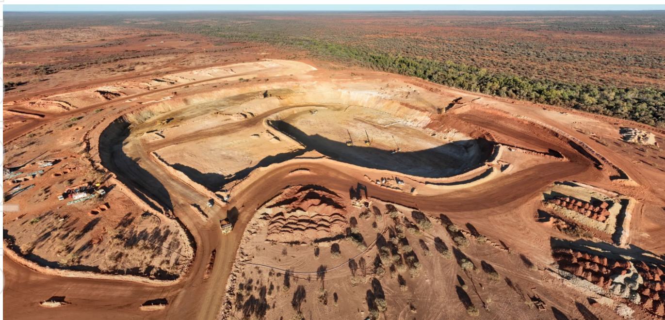
Figure 1: Progression of Stage 1 pit inside larger Stage 2 pit boundary
